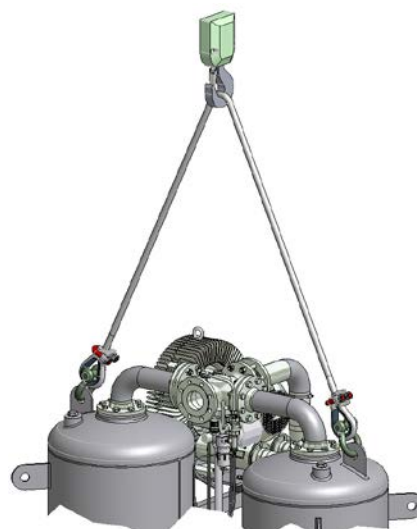
Transport by crane
