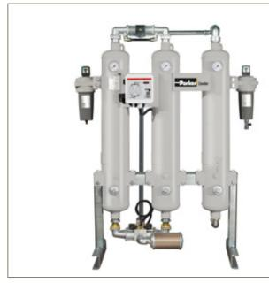
Dry compressed air then enters the integral activated carbon purifier stage, where oil-vapour and odour is reliably removed. Finally, the clean, dry air exits via the validated GL after-filter, into the downstream compressed air network.
