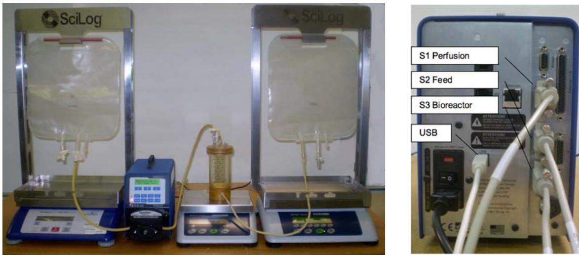
1. Position the Bioreactor, Exact Feed MabTec and the Feed scale in close proximity to each other, keeping cabling, tubing, and replacement of the Feed vessel in mind.
