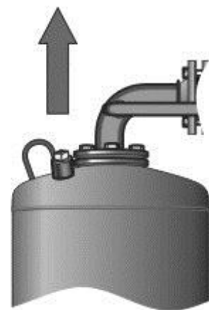
Eyebolt at vessel
