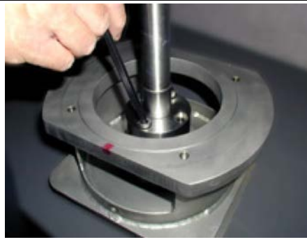
Photo 11: Two allen head cap screws hold the idL™ bearing seal in place.
