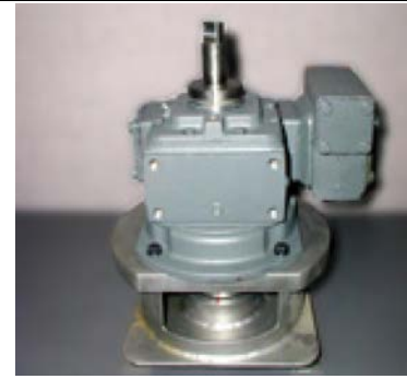
Photo 12: After the idL™ bearing seal is in place, the gear reducer is replaced on the top of the strainer.
